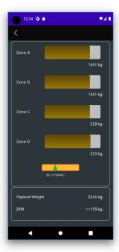
There are four cargo zones in the plane. Drag the slider representing a particular zone from left to right to determine the cargo weight for this zone. The panel also displays the estimated Take-off MAC% which is automatically adjusted while you load cargo in each zone. If the estimated MAC% is outside of allowed limits, it becomes highlighted in red.
