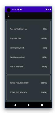
Amount of fuel impacts the center of gravity of the plane. As in the case with loading passengers, the Application estimates the take-off MAC% with the current fuel load.
