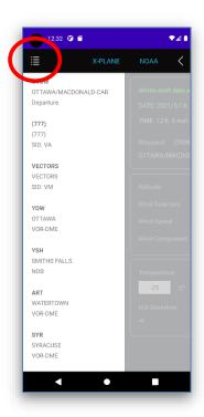
Wind direction, speed, and temperature can also be manually edited for each waypoint in the flight plan. The edited information will be applied only to the selected waypoint.
