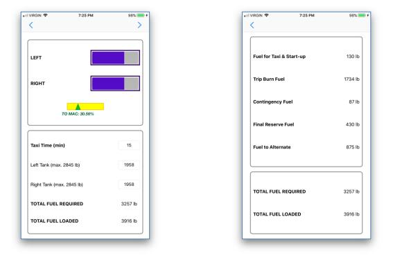
Amount of fuel impacts the center of gravity of the plane. As in the case with loading passengers, the Application estimates the take-off MAC% with the current fuel load.
