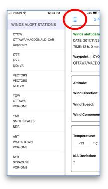
Wind direction, speed, and temperature can also be manually edited for each waypoint in the flight plan. The edited information will be applied only to the selected waypoint.
