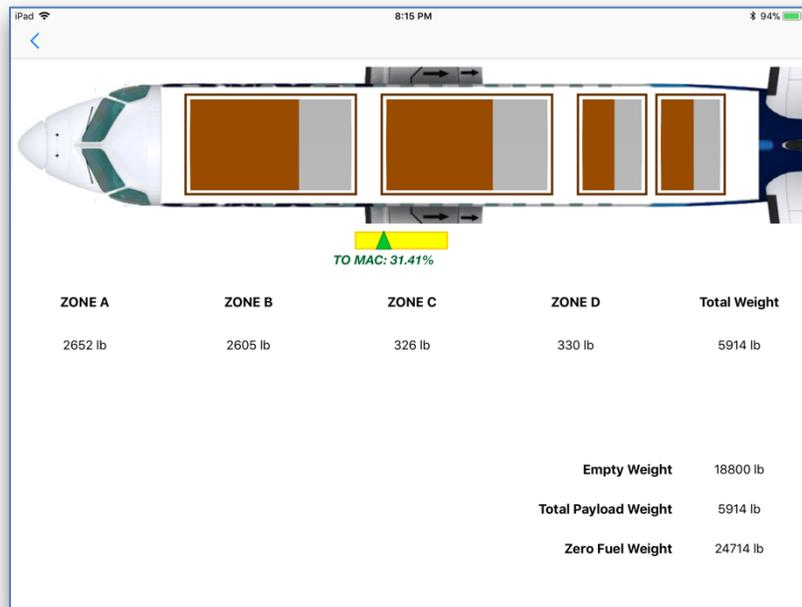
There are four cargo zones in the plane. Drag the slider representing a particular zone from left to right to determine the cargo weight for this zone. The panel also displays the estimated Take-off MAC% which is automatically adjusted while you load cargo in each zone. If the estimated MAC% is outside of allowed limits, it becomes highlighted in red.
