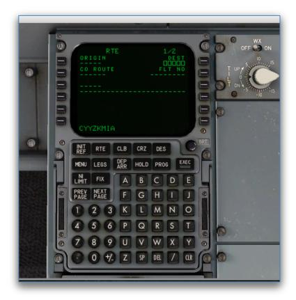
A file with the same name was to be saved in the coroute folder of your plane. If the file is found and does not contain any errors, the co-route is loaded and can be activated.
